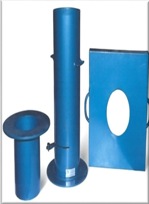
SAND REPLACEMENT METHOD
